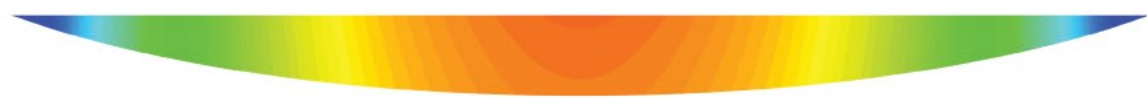
Tensile Membrane Stress diagram showing relatively modest stress levels; greatest at center and least at ends.
